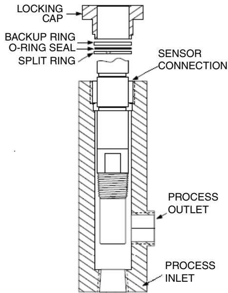
**Ball Valve Insertion Assembly (BVA)**
