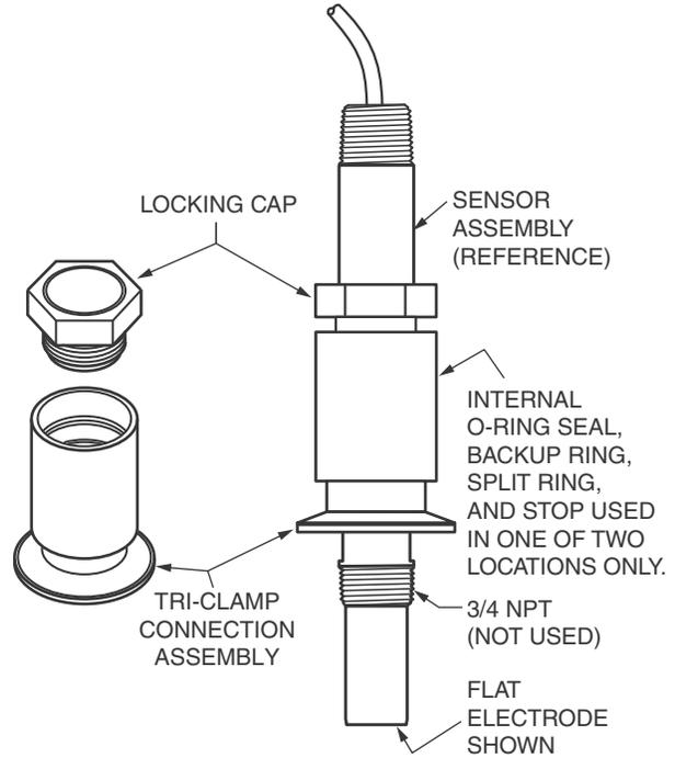
**Flanged Mounting Kits with Integral (Welded-in-Place) Universal Bushing Assembly**
