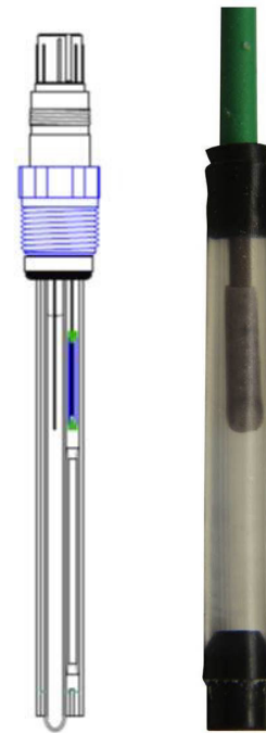
Figure 3. This cutaway view of the Foxboro PH12 sensor shows the unique, long-life design of its double junction solution reference.
