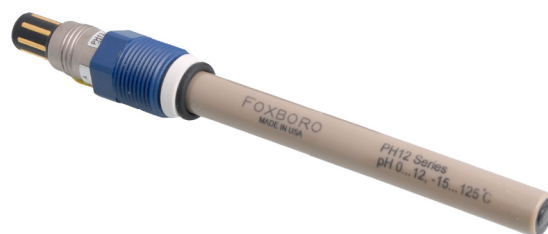
Figure 1. Improving pH sensor durability demands innovations to reduce the risk of breakage while preserving the cleanability, selectivity, and performance associated with glass bodies and dome-style glass electrodes. The Foxboro PH12 family of 3-A Sanitary compliant pH sensors incorporates a durable PEEK body with a specially engineered, ruggedized flat-glass electrode.
