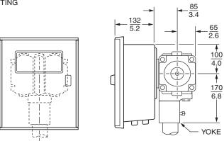
MOUNTING WITH A TYPE 37 DIFFERENTIAL PRESSURE ELEMENT
